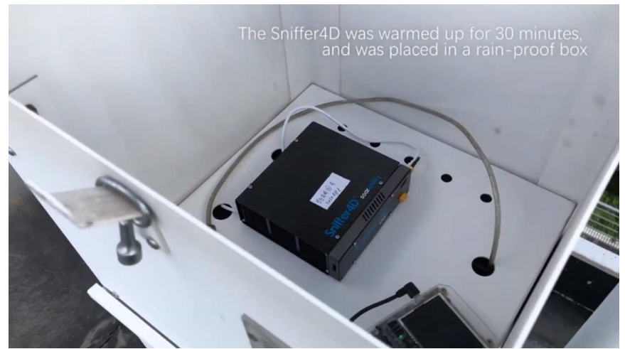
The Sniffer4D was warmed up for 30 minutes, and was placed in a rain-proof box
