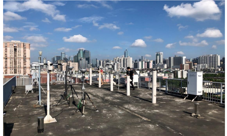
The Sniffer4D was warmed up for 30 minutes, and was placed in a rain-proof box
